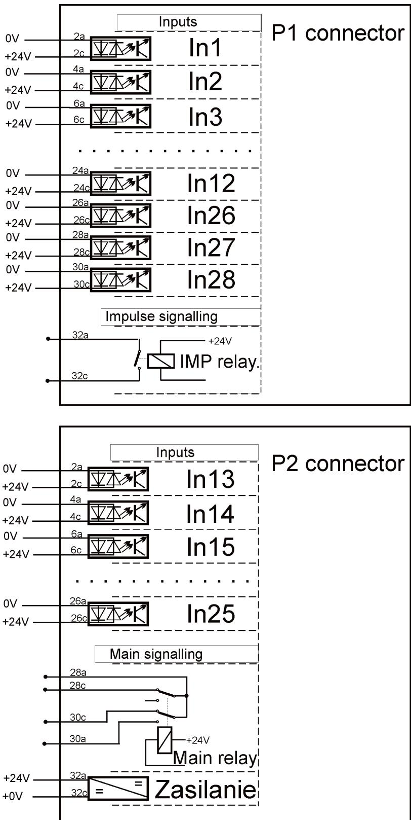
Fig. 5. Description of P1 and P2 connectors.
