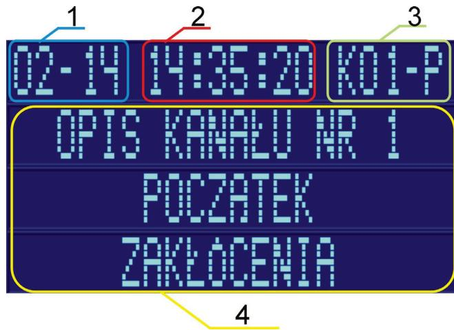
Fig. 2. LCD display view – alarm notification.
