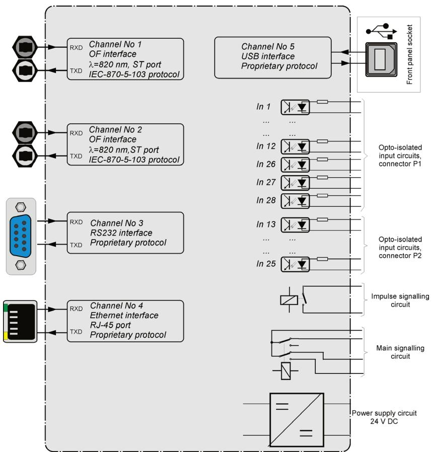
Fig. 1. Flowchart of a ZRZ-28 recorder
