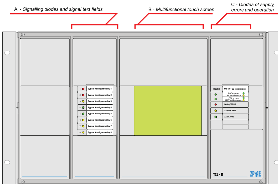
Fig. 3. Layout of a TSL-11 unit (standard version).
