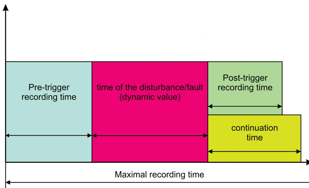
Fig. 3.1. Record time diagram
