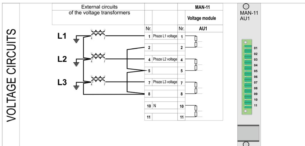
Fig. 3.3. Voltage circuits.
