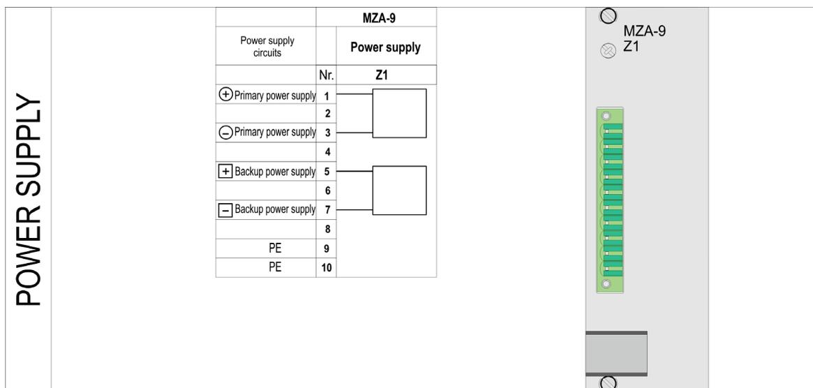
Fig. 3.7. Recorder power supply.
