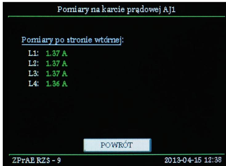
Fig. 2.9. Preview screen with current measurements from analogue inputs.
