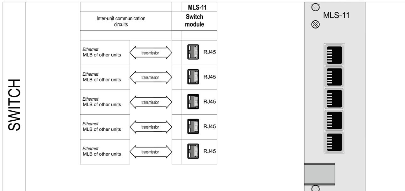
Fig. 3.9. Optional switch module after connection to a distributed RZS-9 system.
