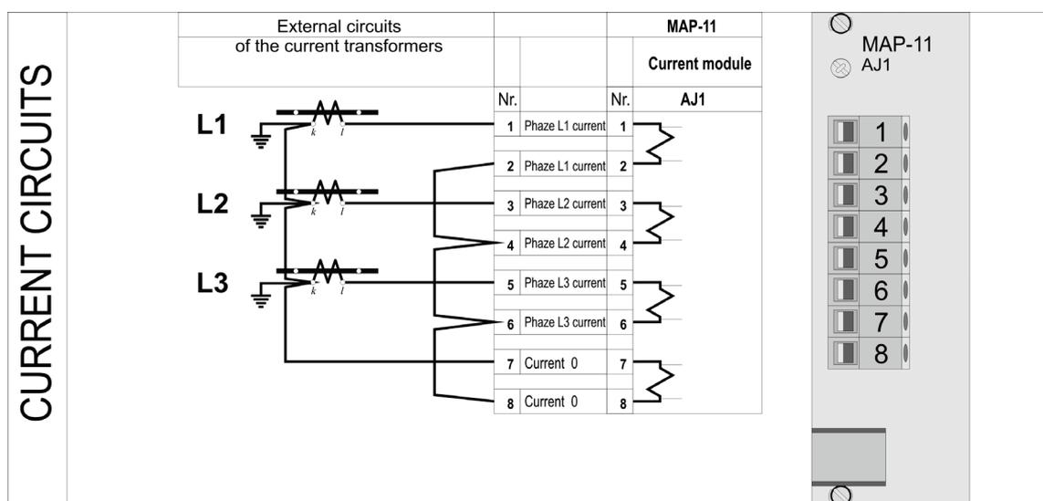
Fig. 3.4. Current circuits.
