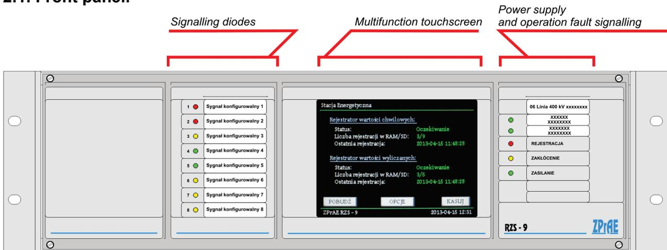
Fig. 2.2. Front panel.
