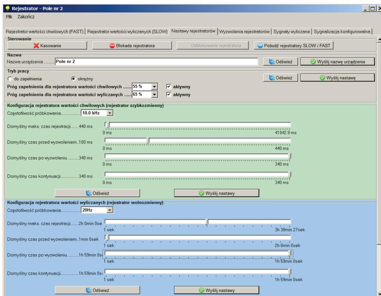
Fig. 4.11. Recorder setups window.
