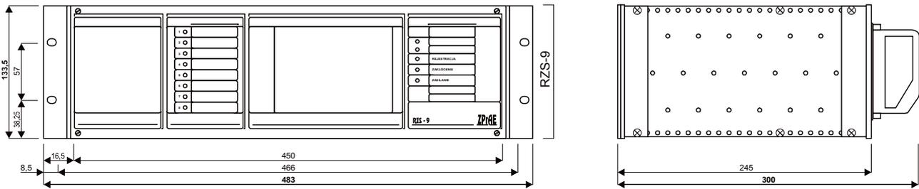
Fig. 2.1. External dimensions of the recorder.
