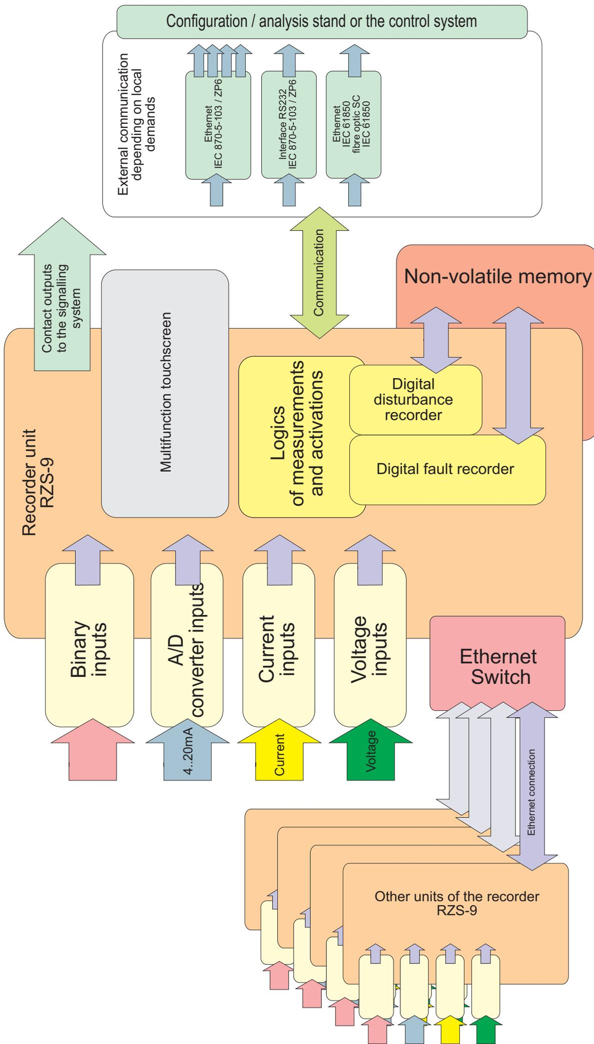
**Structural diagram of the disturbance recorder RZS-9**
