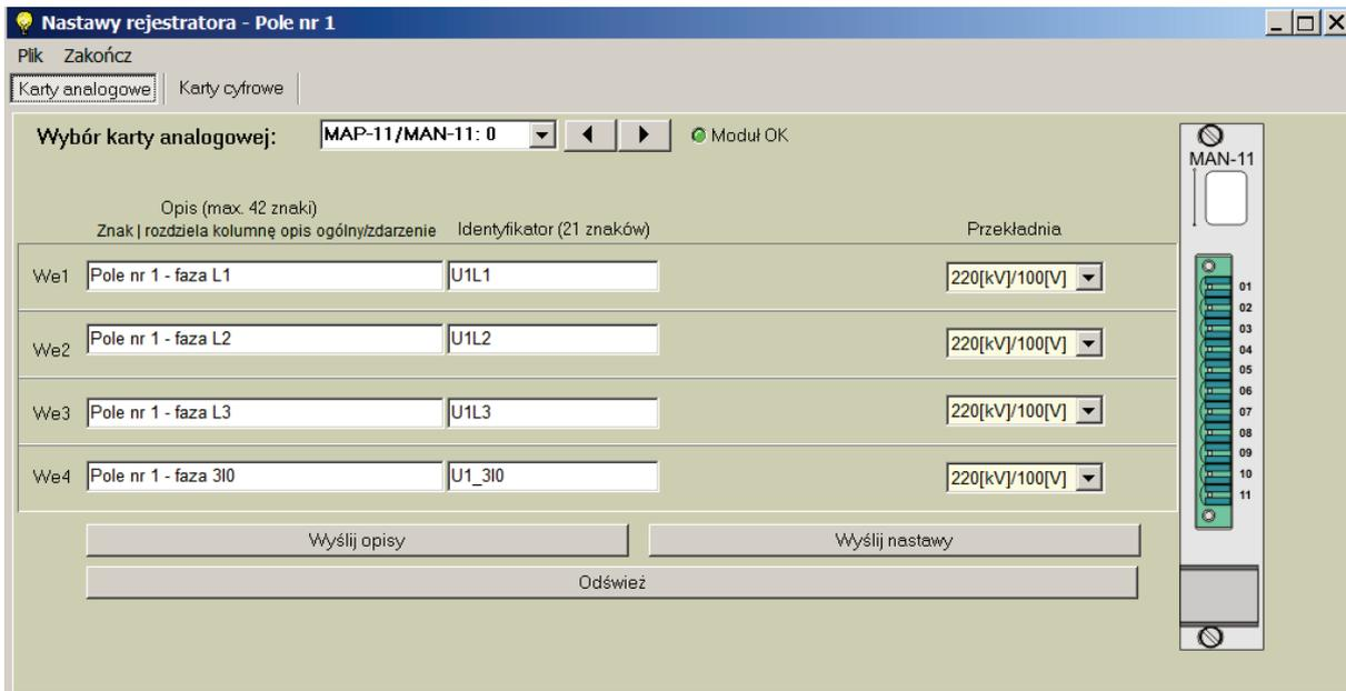
Fig. 4.7. Analogue card setup window.
