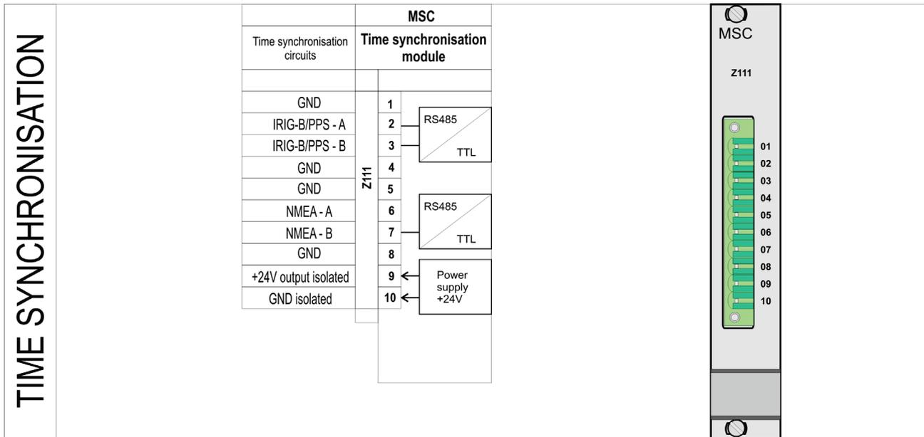
Fig. 3.2. MSC-11 time synchronization module.
