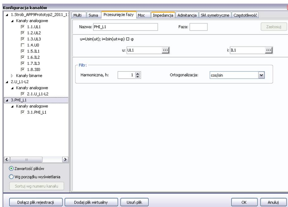
Fig. 5.4.  $PHI_{L1}$  virtual channel configuration
