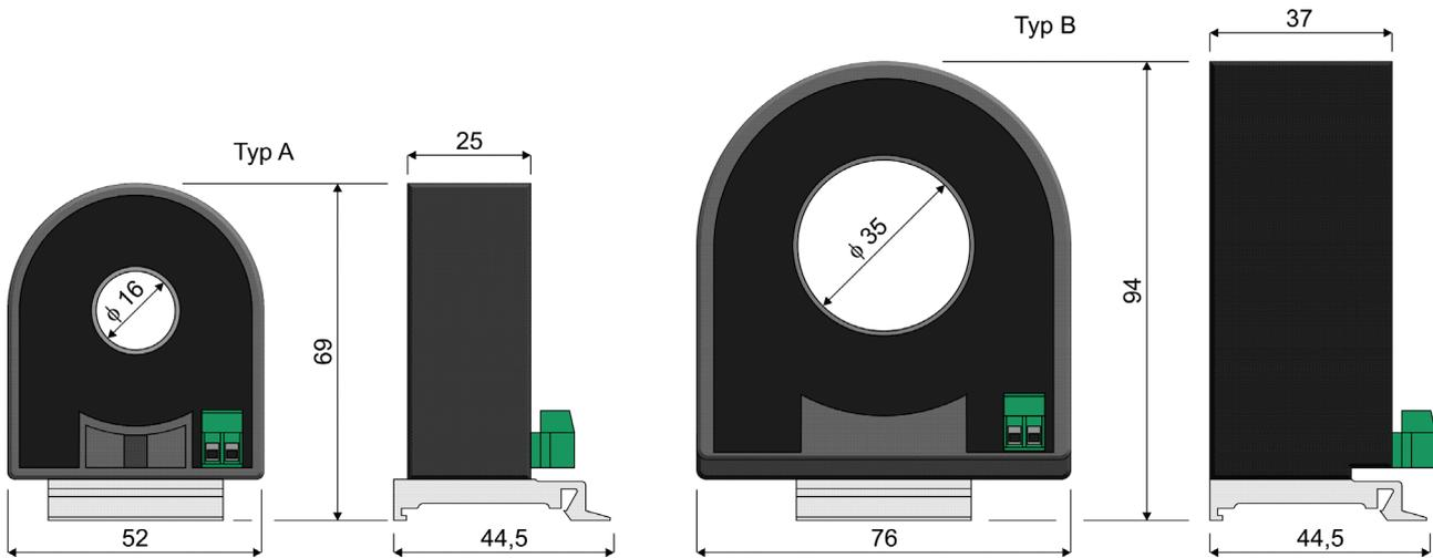
Fig. 6.2.1. Dimension drawing of the KDZ-3PP Type A instrument transformer.
