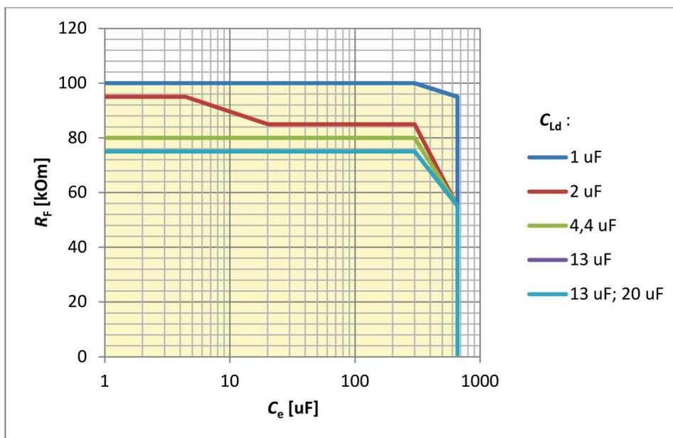
Graph 11.6. Range of allowable earth fault resistance for which the locating unit will locate the earth fault correctly as a function of system capacitance  $C_e$  including capacitance after the measuring transformer  $C_{Ld}$  for network voltage of 48 V DC. Measured resistance may exceed the declared measurement error.
