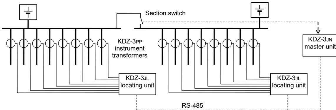
Fig. 3.2.3. Structure of the KDZ-3 earth fault monitoring system in a two-section switchgear with one master unit.
