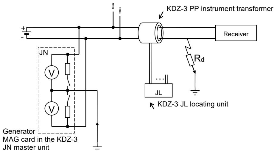
Fig. 3.1.2. Concept of generator's operation.
