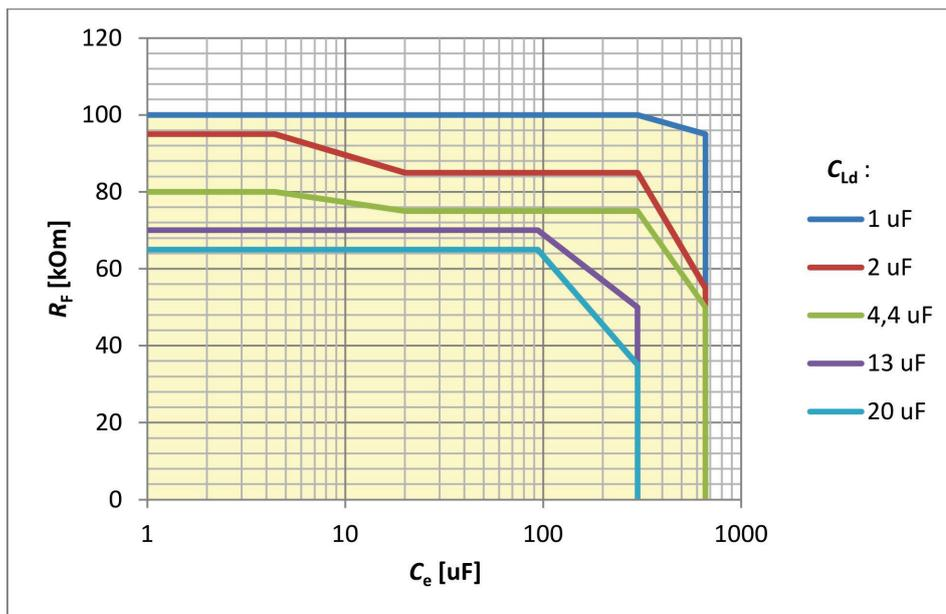
Graph 11.5. Range of allowable earth fault resistances for which the locating unit will locate the earth fault and measure the resistance correctly with a declared error as a function of system capacitance  $C_e$  including capacitance after the measuring transformer  $C_{Ld}$  for network voltage of 48 V DC.
