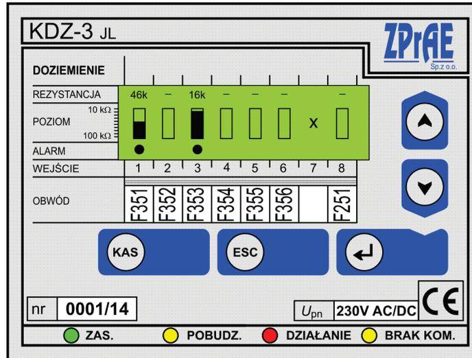
Fig. 5.1.1. View of the front panel of the KDZ-3JL locating unit.
