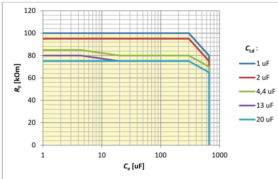
Graph 10.4. Range of allowable earth fault resistance for which the locating unit will locate the earth fault correctly as a function of system capacitance  $C_e$  including capacitance after the measuring transformer  $C_{Ld}$  for network voltage of 110 V DC. Measured resistance may exceed the declared measurement error.
