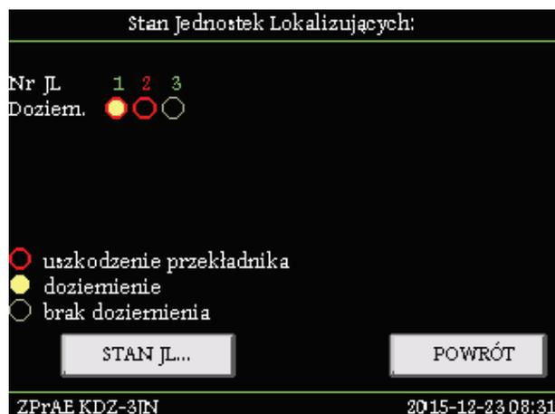
Fig. 4.3.5. Screen with current status of locating units.
