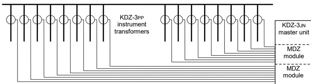
Fig. 3.2.2. Centralized version of the KDZ-3 earth fault detection system.
