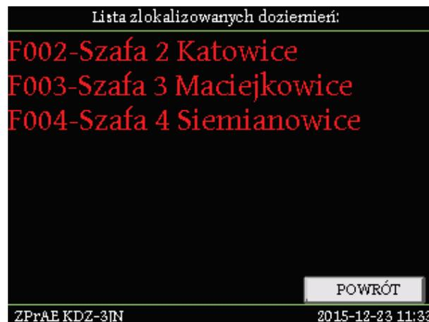
Fig. 4.3.4. List of outgoing feeders with earth faults.
