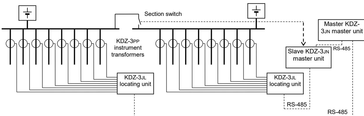
Fig. 3.2.4. Structure of the KDZ-3 earth fault monitoring system in a two-section switchgear with two master units.
