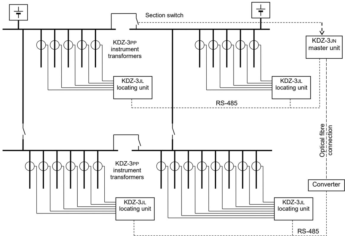
Fig. 3.2.5. Structure of the KDZ-3 earth fault monitoring system with the following setup: two-section main switchgear and a sub-switchgear.
