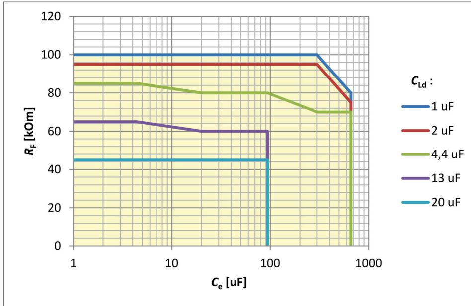
Graph 11.3. Range of allowable earth fault resistances for which the locating unit will locate the earth fault and measure the resistance correctly with a declared error as a function of system capacitance  $C_e$  including capacitance after the measuring transformer  $C_{Ld}$  for network voltage of 110 V DC.
