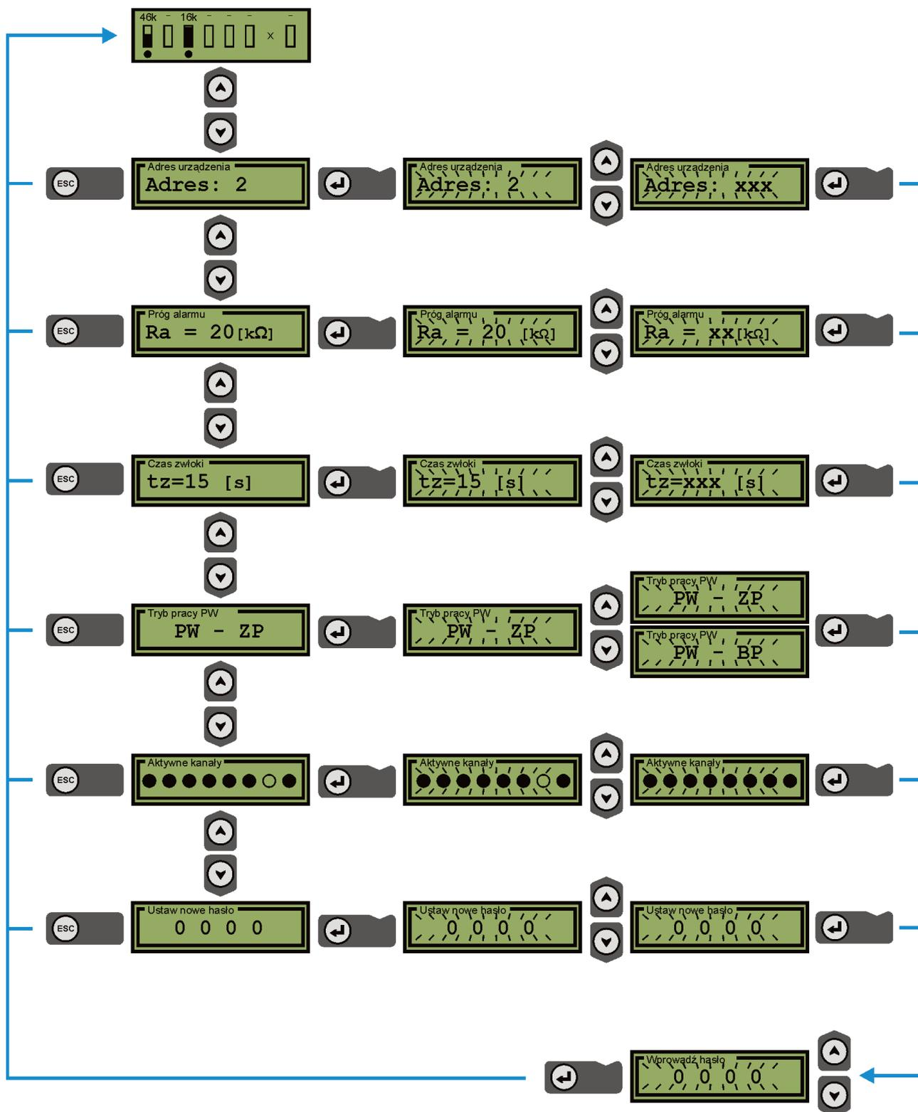
Fig. 5.3.2. Flowchart of parameter preview and configuration.
