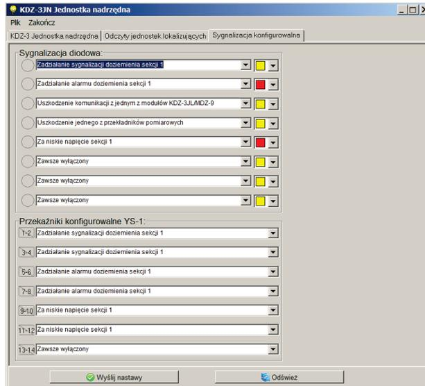
Fig. 9.7. Signaling configuration window.
