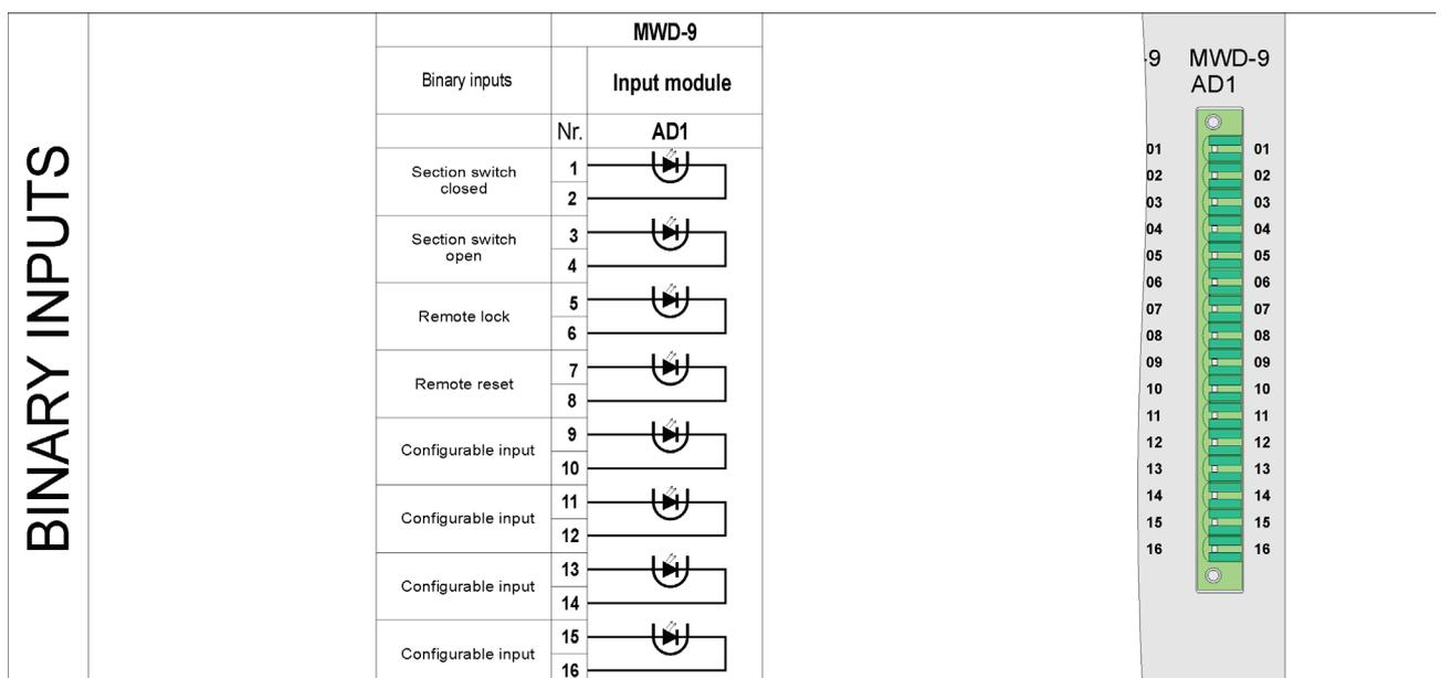
Fig. 4.4.4. Binary inputs of the MWD-9 module.
