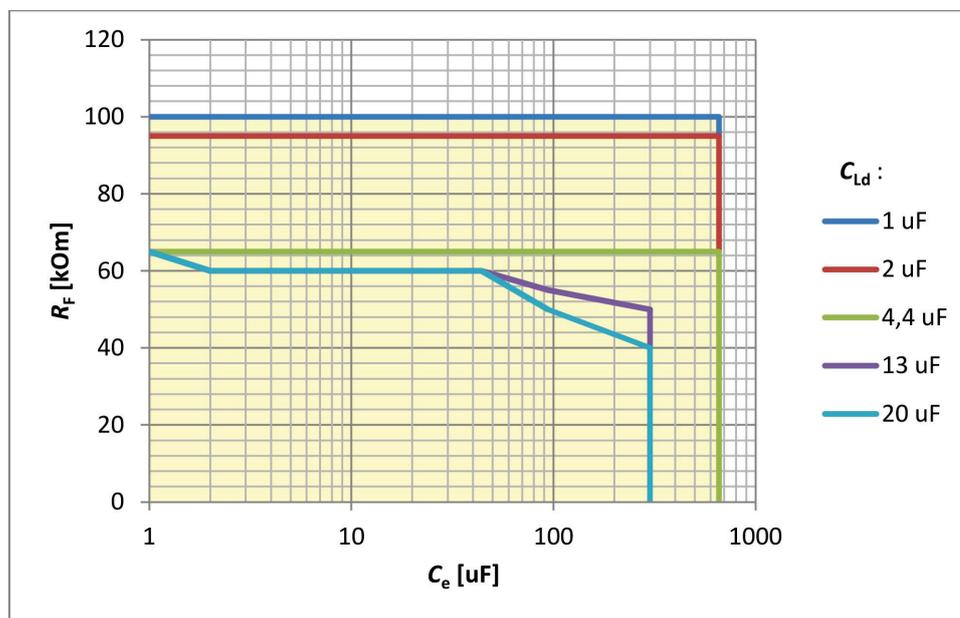
Graph 11.2. Range of allowable earth fault resistance for which the locating unit will locate the earth fault correctly as a function of system capacitance  $C_e$  including capacitance after the measuring transformer  $C_{Ld}$  for network voltage of 220 V DC. Measured resistance may exceed the declared measurement error.
