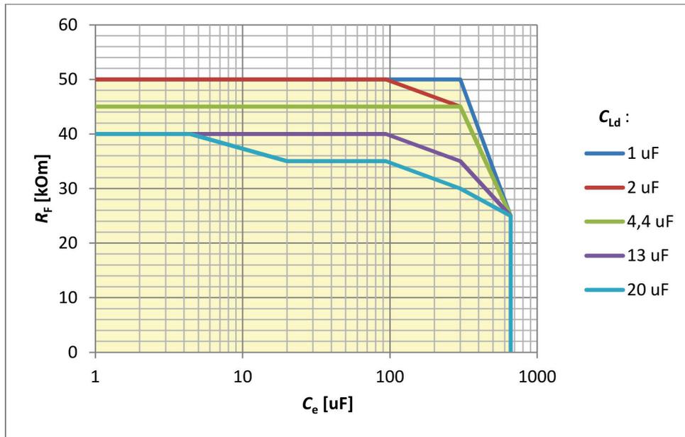
Graph 11.7. Range of allowable earth fault resistances for which the locating unit will locate the earth fault and measure the resistance correctly with a declared error as a function of system capacitance  $C_e$  including capacitance after the measuring transformer  $C_{Ld}$  for network voltage of 24 V DC.
