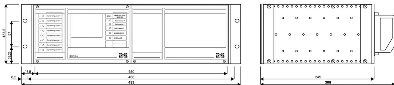
Fig. 4.2.1. External dimensions of the KDZ-3JN master unit.
