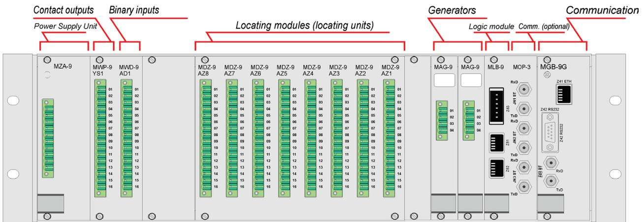
Fig. 4.4.2. Rear panel of version E of the KDZ-3JN master unit (with MDZ modules fulfilling the role of locating units).
