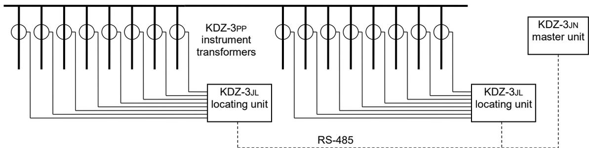
Fig. 3.2.1. Structure of the KDZ-3 distributed earth fault detection system.
