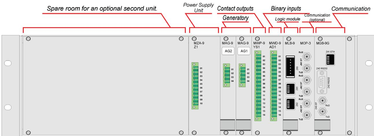
Fig. 4.4.1. Rear panel of version E of the KDZ-3JN master unit.
