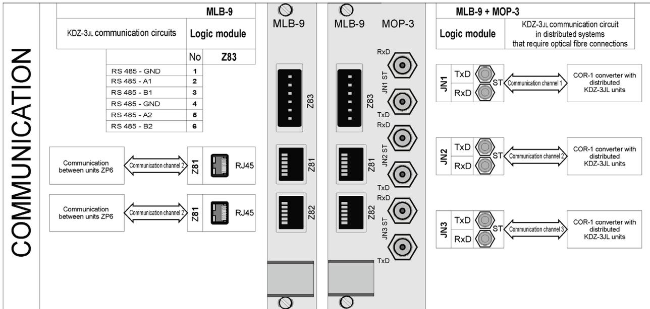
Fig. 4.4.7. Communication with locating units.
