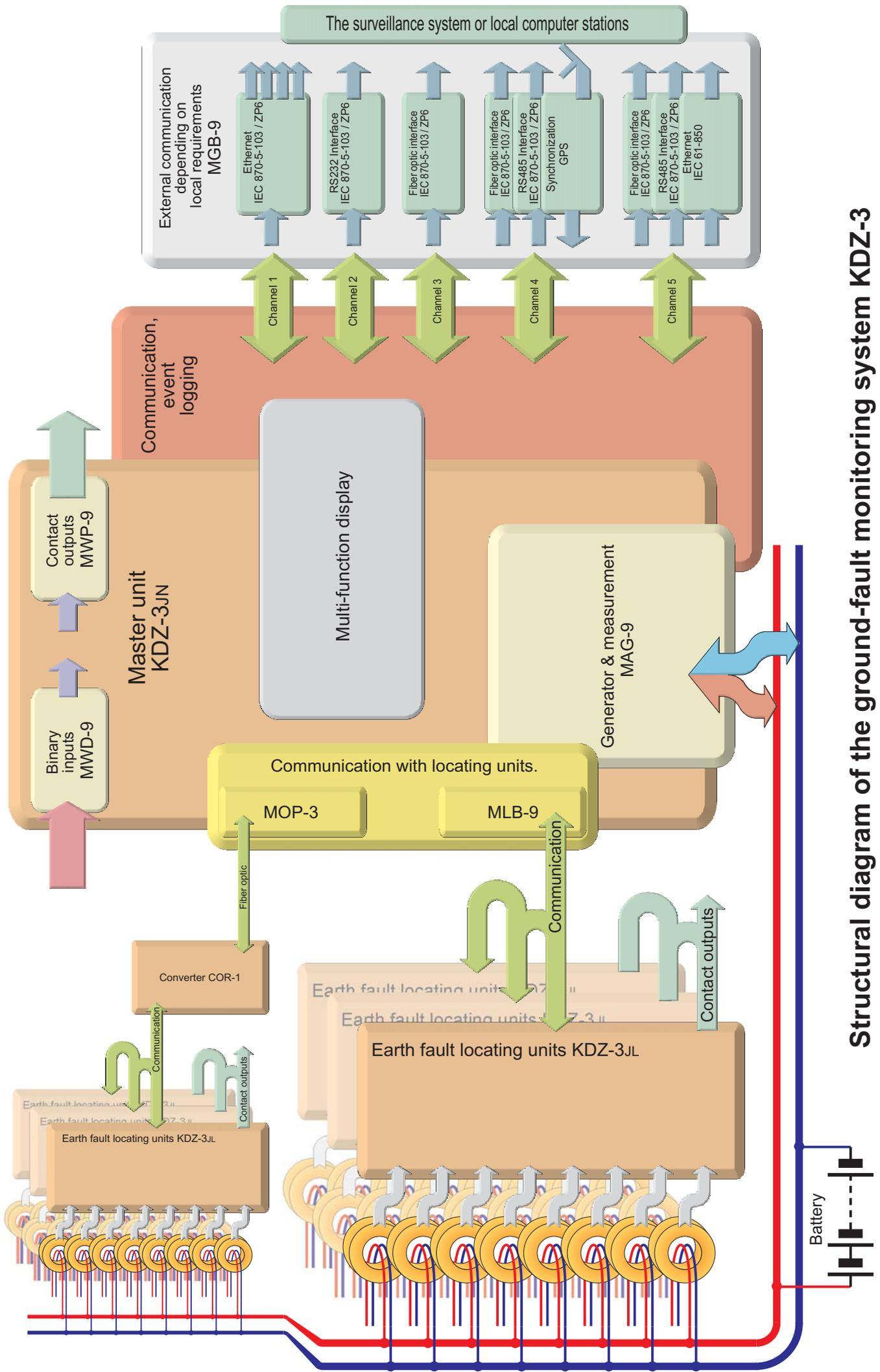
Structural diagram of the ground-fault monitoring system KDZ-3
