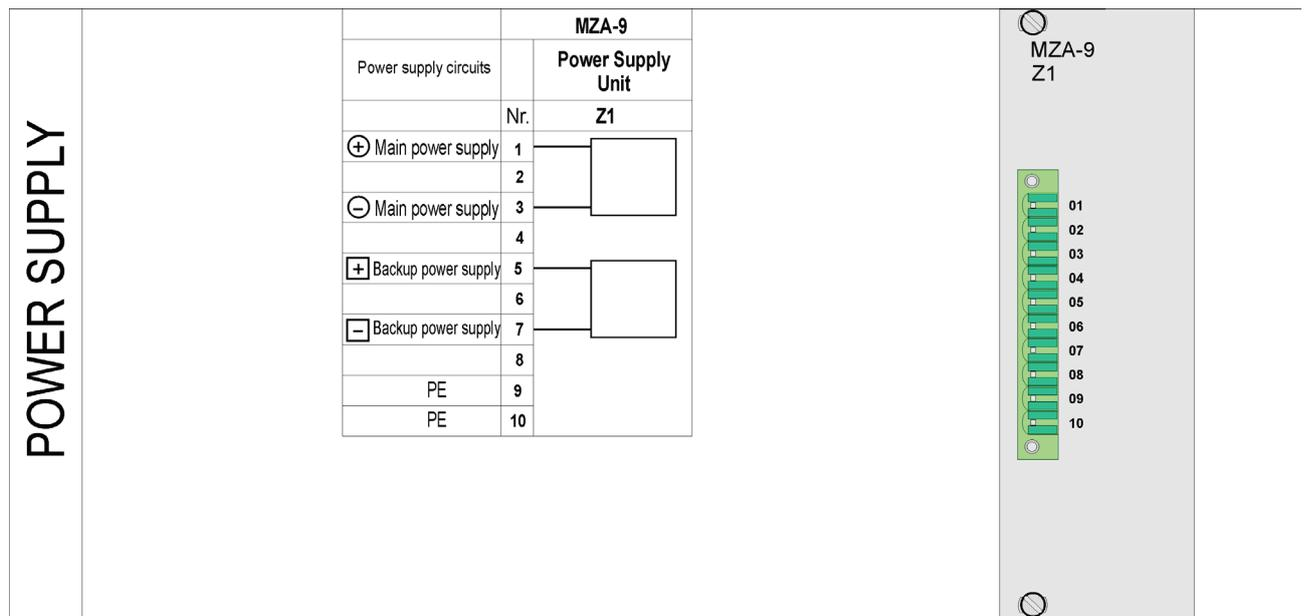
Fig. 4.4.6. MZA-9 power supply unit.
