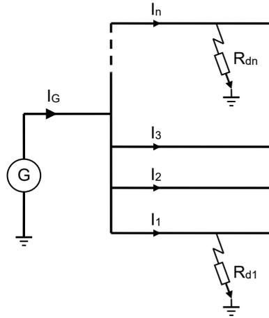
Fig. 3.1.1. Earth fault measurement concept.
