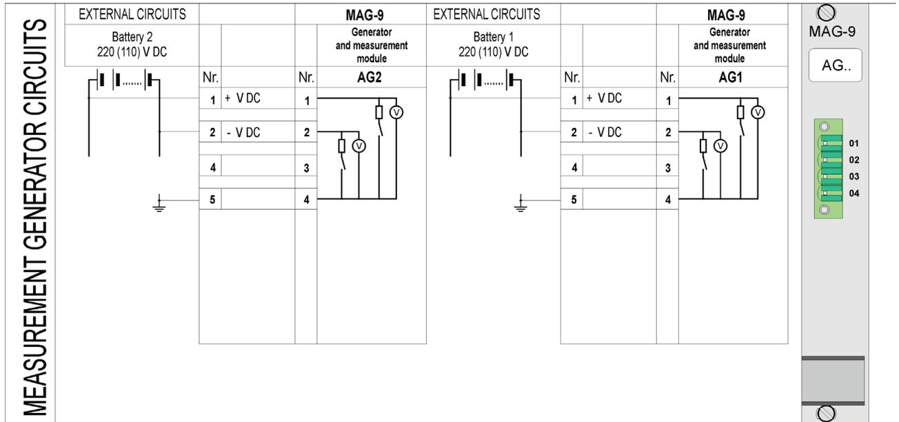
Fig. 4.4.3. Generator and measurement circuits of MAG-9 modules.
