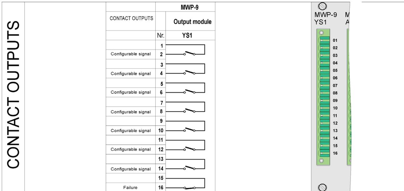
Fig. 4.4.5. Contact outputs of the MWP-9 module.
