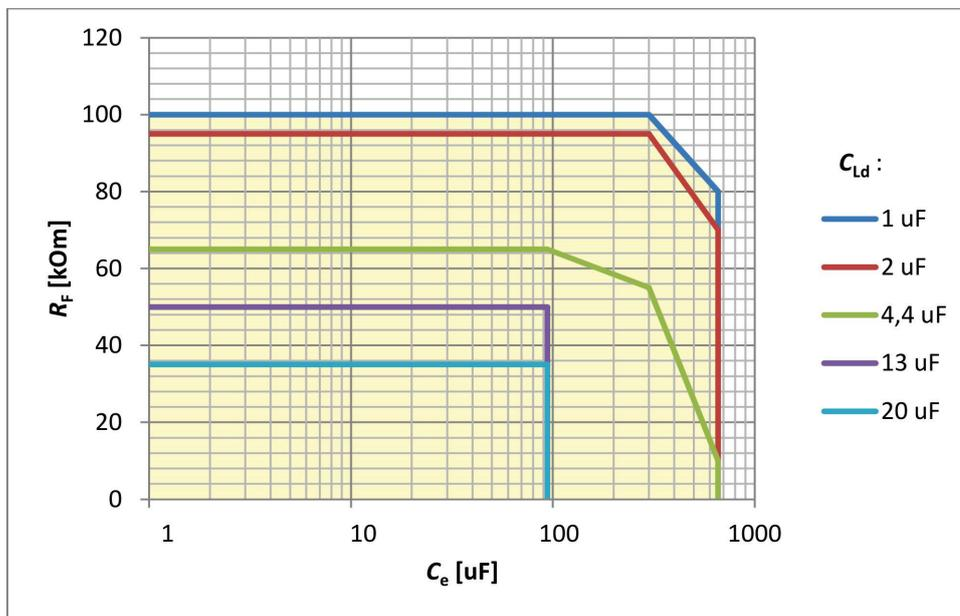
Graph 11.1. Range of allowable earth fault resistances for which the locating unit will locate the earth fault and measure the resistance correctly with a declared error as a function of system capacitance  $C_e$  including capacitance after the measuring transformer  $C_{Ld}$  for network voltage of 220 V DC.
