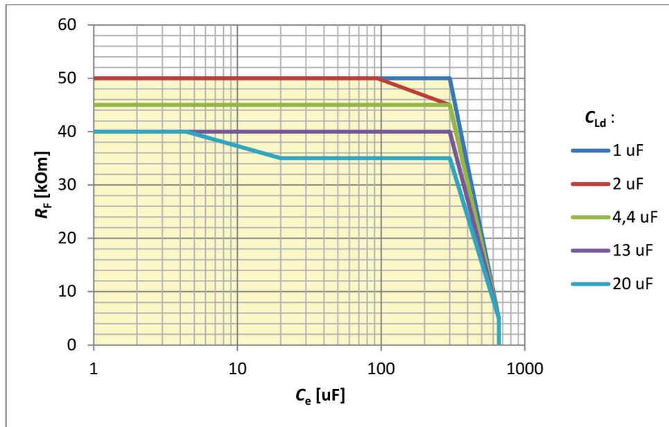
Graph 11.8. Range of allowable earth fault resistance for which the locating unit will locate the earth fault correctly as a function of system capacitance  $C_e$  including capacitance after the measuring transformer  $C_{Ld}$  for network voltage of 24 V DC. Measured resistance may exceed the declared measurement error.
